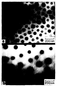
Figure 1 TEM micrographs of P(S-b-2VP) film cast from benzene and stained with methyl iodide: (a) before and (b) after crosslinking
