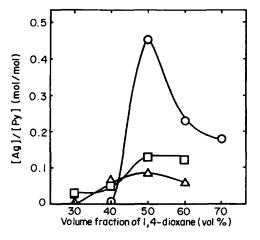
Figure 9 Amount of colloidal silver introduced into the film: ( $\triangle$ ) M1 series; (○) M2 series; (□) M3 series
