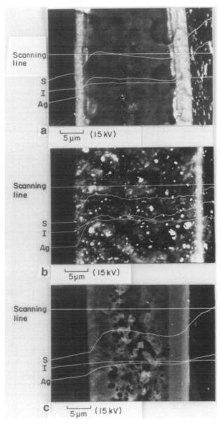
Figure 6 BSE images of the cross-section of the M2 series observed by SEM: (a) M2-50; (b) M2-60; (c) M2-70
