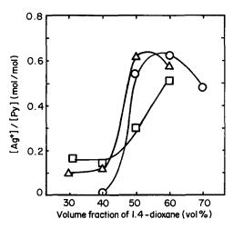
Figure 8 Amount of Ag<sup>+</sup> ion penetrated into the film: ( $\triangle$ ) M1 series; (○) M2 series; (□) M3 series
