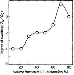
Figure 2 Swelling behaviour of M1 in the water/DIOX system
