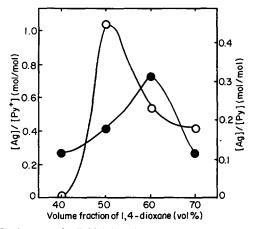
Figure 5 Amount of colloidal silver introduced into the film: ( ) M20 series; (O) M2 series
