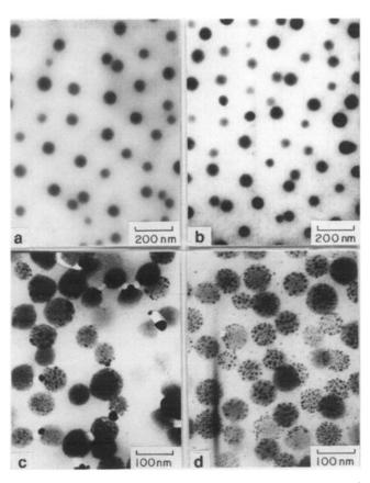
Figure 7 TEM micrographs of M2-50: (a) before soaking in the Ag<sup>+</sup> ion solution; (b) after soaking in the Ag+ ion solution; (c) after chemical reduction; (d) after removing AgI with Na<sub>2</sub>S<sub>2</sub>O<sub>3</sub>
