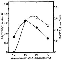
Figure 4 Amount of Ag + ion penetrated into the film: ( ) M20 series; (O) M2 series
